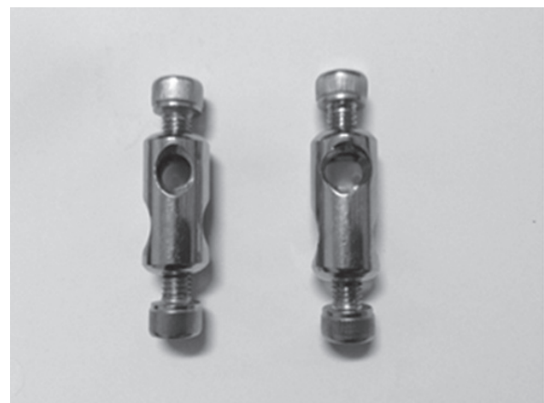
Figure 1 The Old (Left) and New (Right) joint designs of the external fixator
