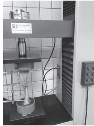
Figure 4 The compression mode test machine and the specimen
