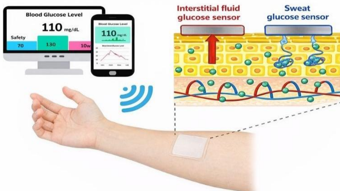
Figure 6 Example of Non-invasive Epidermal Glucose Sensors (18)
